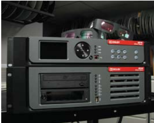
The Guild's new Dolby Digital Cinema Servers with Dolby 3-D conversion kits
